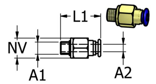
Ext. hose diameter A2 = 4 mm L1 = 17.5 NV = 8 Thread A1 = M3
